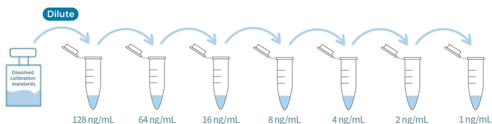
Figure 3. Graphic scheme of CHO HCP Calibration Standard Solutions
